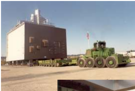
Pic. 23 Goldhofer THP/H 24 P with 1.200 t module
