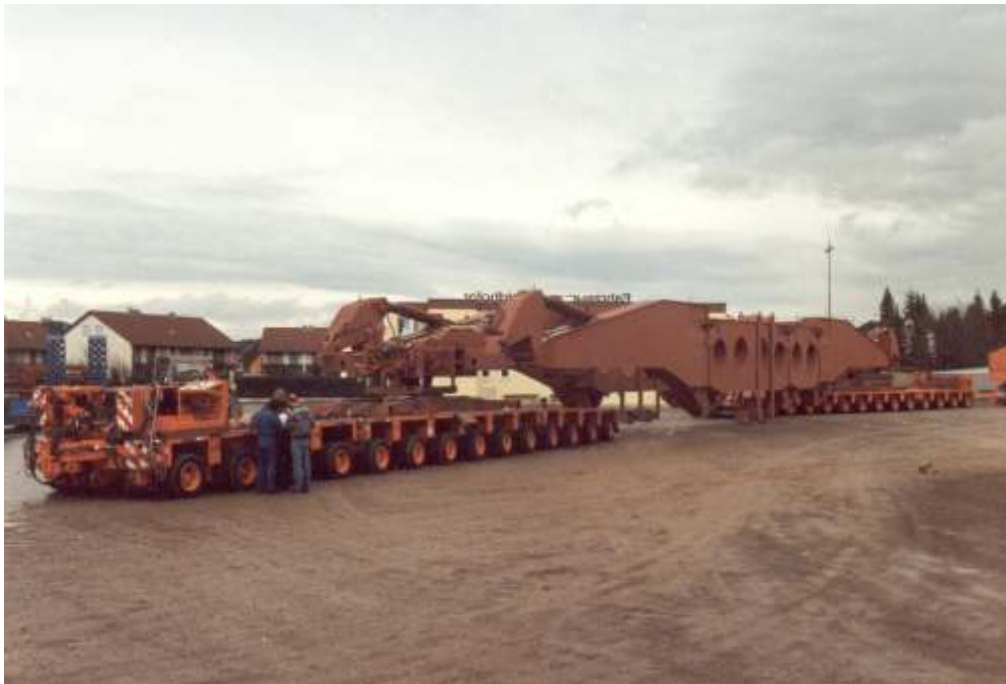
Pic. 37 girder frame trailer with max. payload of 385 t on test ride at Goldhofer company in Memmingen
