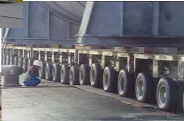
Pic. 35 impressive: the hydraulic axleload compensation
