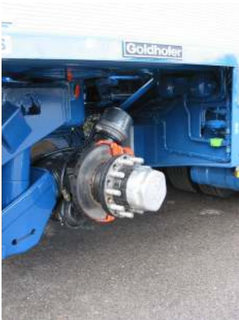
Pic. 56 THP/UT with air-operated disc brakes
