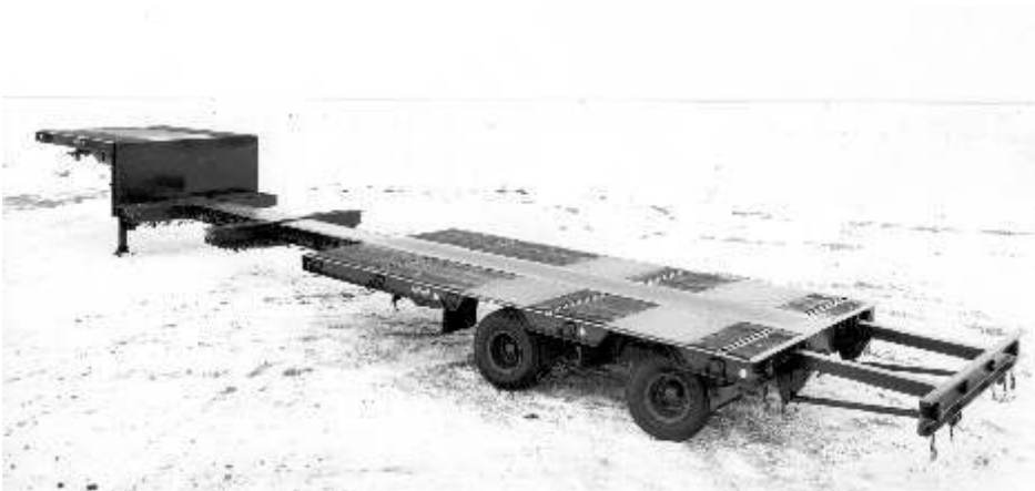
Pic. 14 the first extendible Goldhofer Lowbed-Semitrailer
