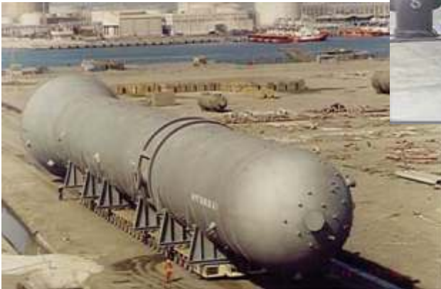
Pic. 34 the 800t load on a modular tractor / trailer unit
