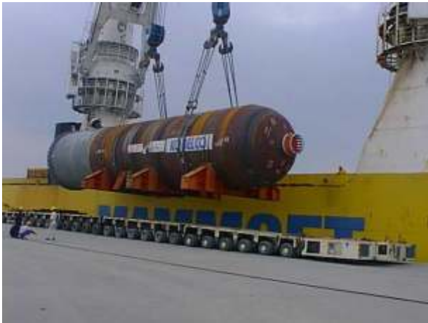
Pic. 36 first selfpropelled module, coupled with trailer modules
