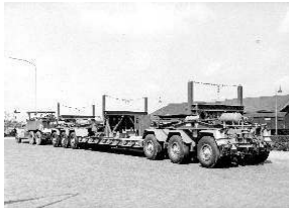
Pic. 9 ... a Goldhofer lowloader TA6 with a permissible gross weight of 120 t
