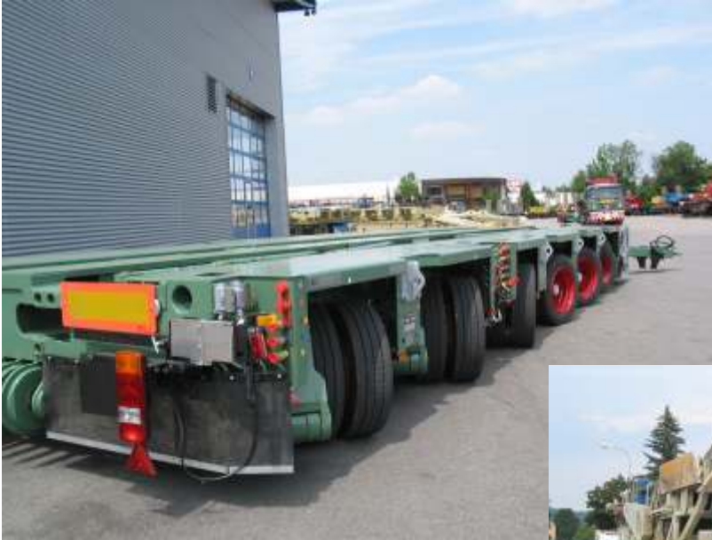
Pic. 52 THP/UT platform modules with two and four axle lines are combined to form a six-axle trailer
