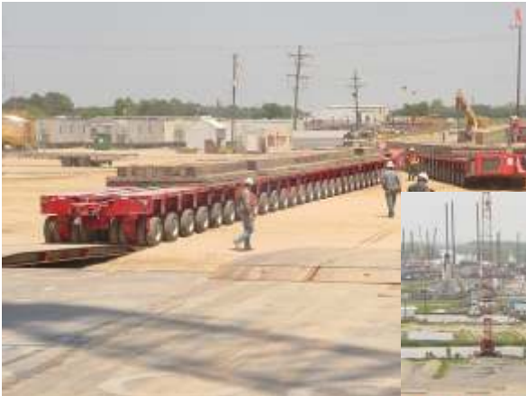
Pic. 60 PSP module transporter prepared for the next load
