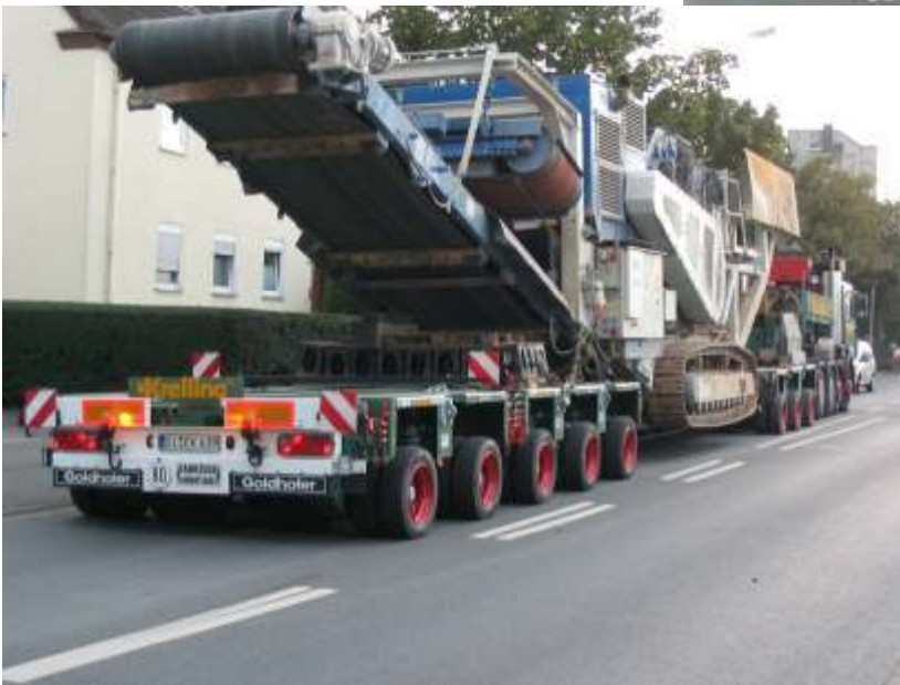
Pic. 54 THP/UT platform modules with two and three axle lines in a semitrailer combination
