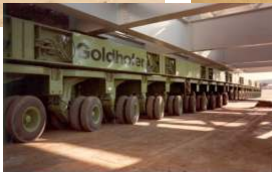
Pic. 24 These vehicle dimensions can only be realized by means of an hydraulic axle load compensation
