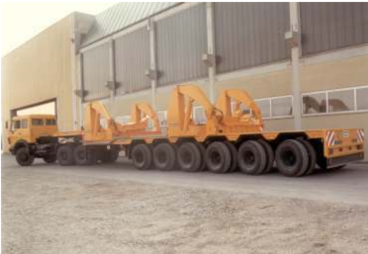
Pic. 27 SKPH 6 with huge 11.00-20 tyres and lifting device for a 55 tons telescopic derrick boom of a Gottwald mobile crane type AMK 600
