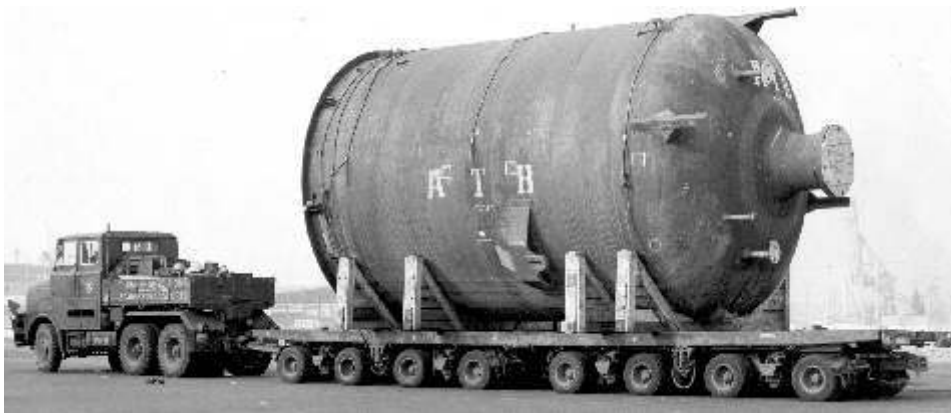
Pic. 11 TPA8 with vessel (D 6 m L 13 m weight 160.000 kg)
