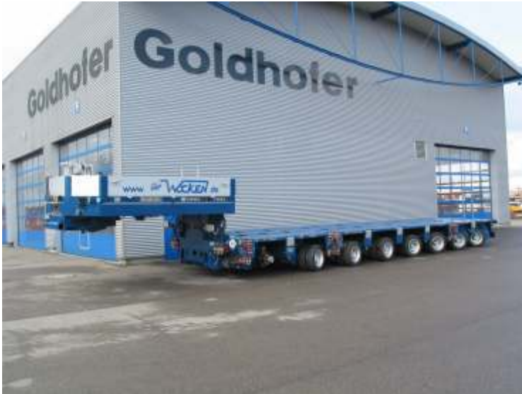
Pic. 55 THP/UT platform modules with 2 + 4 + 2 axle lines are combined to form an eight-axle semitrailer
