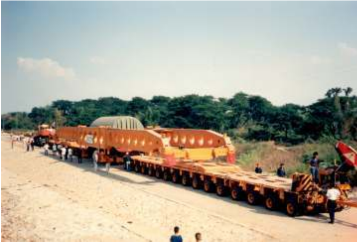
Pic. 28 girder frame on two THP/LV 16-axlelines modular trailers
