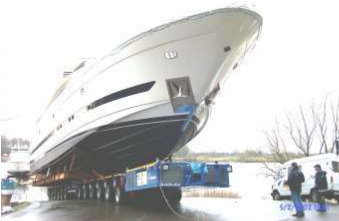
Pic. 51 Operation of the new self-propelled module for transporting the yacht "Elegance"
