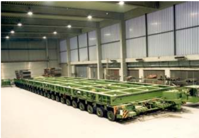
Pic. 25 THP/H 24 side-by-side combination in Memmingen ready for final inspection by customer
