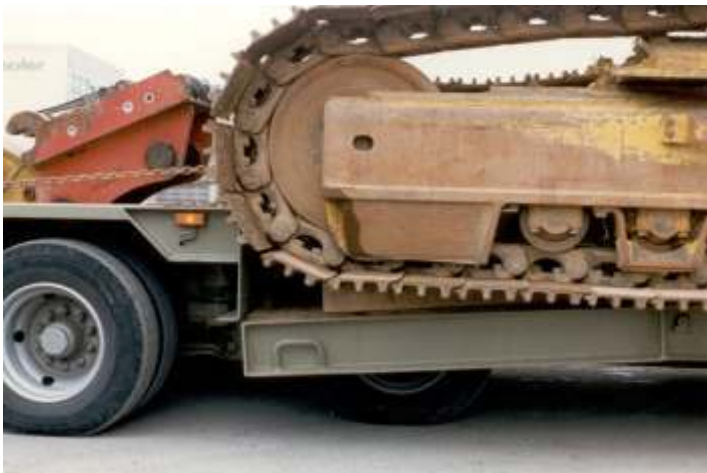
Pic. 42 Narrow track axle between the tracks of an excavator
