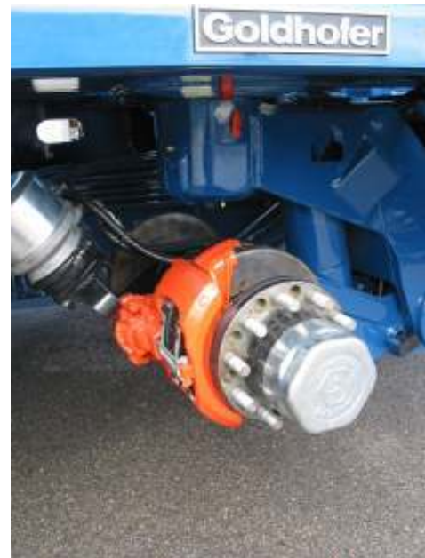
Pic. 57 THP/UT with air-operated disc brakes
