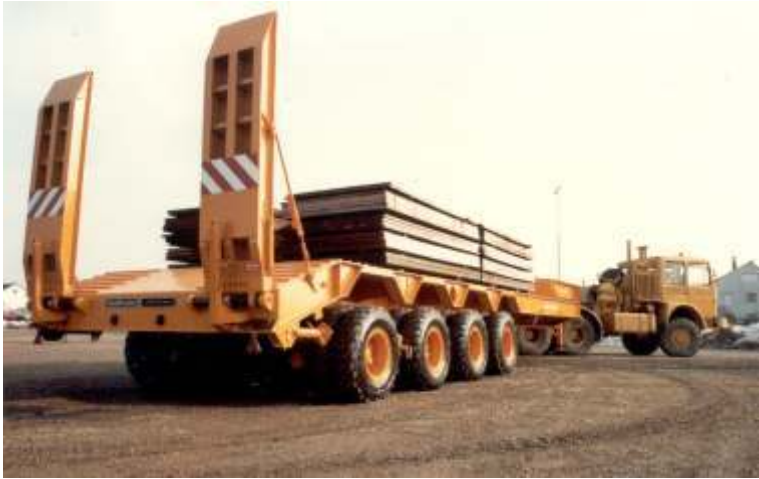
Pic. 26 STUE4 payload rated at 100 t for unpaved ways
