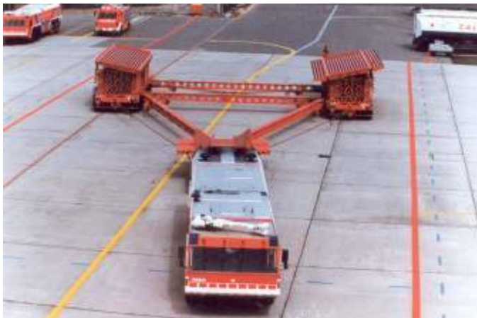
Pic. 32 ARTS (Aircraft Recovery and Transportation System) on duty in Frankfurt
