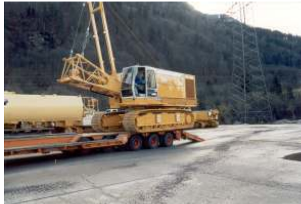
Pic. 41 2 narrow track axles positioned in front of 3 steering axles
