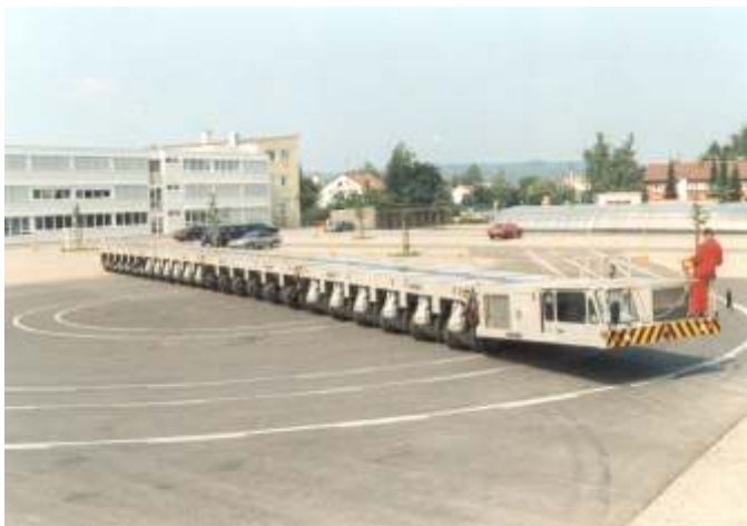
Pic. 39 Four heavy-duty modules coupled one after the other with 24 axle lines
