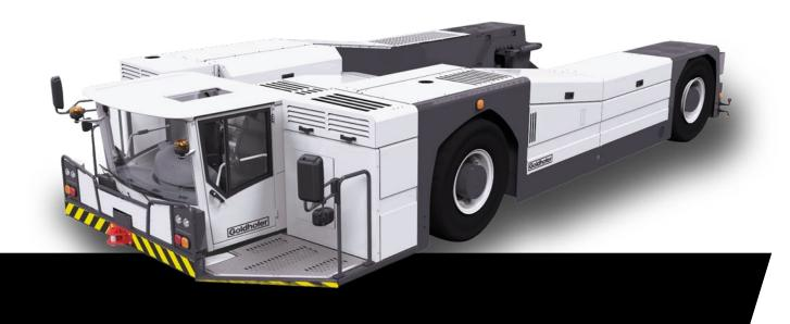
**AST-1X 530** 390 kW | MTOW ≤ 600 t **AST-1X 707** 520 kW | MTOW ≤ 600 t
