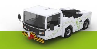
»BISON« E 370  $75 \,\text{kW} \mid 105 \,\text{kN} \mid \text{MTOW} \le 125 \,\text{t}$ 80 kWh | 120 kWh | 160 kWh
