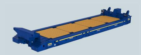
Goldhofer vessel decks can be configured and converted in several different ways for optimal transport conditions.
