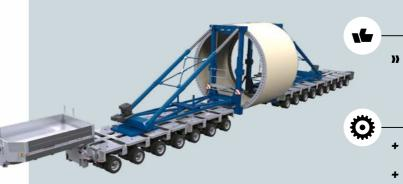
Simple assembly on towed modules guarantees high flexibility for the transport of tower segments and simplifies route planning with FTD.
