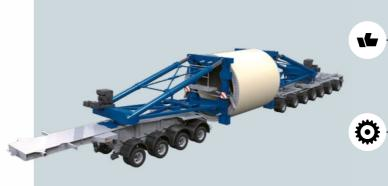
Simple assembly on towed modules guarantees high flexibility for the transport of tower segments and simplifies route planning with FTD.
