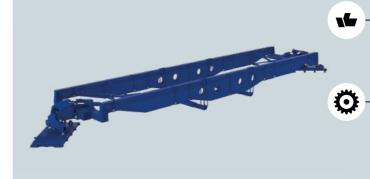
The »FAKTOR« 5 high girder bridge, weighing just 100 t, combines low loading height and optimal load distribution with a maximum load capacity of impressive 500 t.
