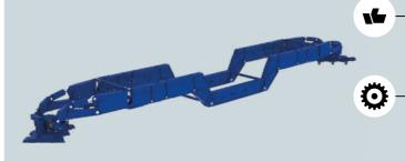
With a payload of 350 t, the »FAKTOR« 5.5 high girder bridge can take on and transport up to 5,5 times its dead weight.
