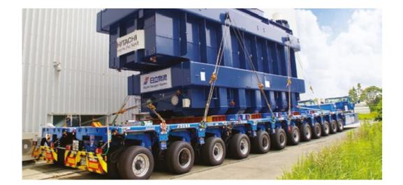
440 t IN JAPAN A parallel combination created with 2x12 axle PST/ES-E moves a generator.
