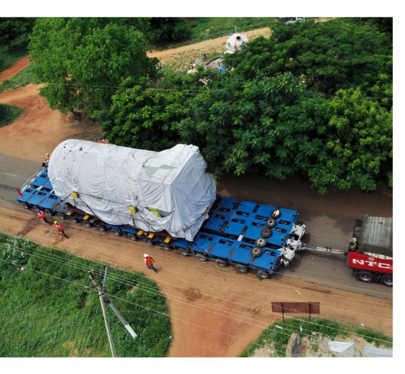
**BEST PERFORMANCE CAPABILITY FOR ANY LOAD**Due to the extensive range of accessories, the THP/SL heavy-duty modules can be flexibly adapted to the specifications of the load, as shown here with a parallel combination (1+1/2).
