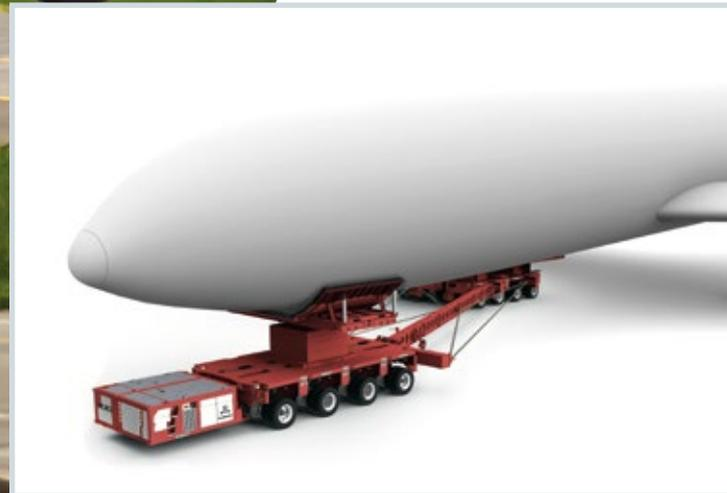
**Increase the risk coverage by adding a wing support module to the front module of the professional or premium solution. This system allows you to recover aircraft with a damaged nose landing gear and one damaged main landing gear.**
