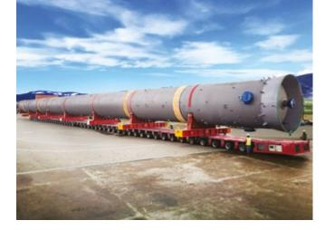
**EXTREME FLEXIBILITY – UNLIMITED POSSIBILITIES** Due to the possibility of combination with other heavy-duty modules, enormous axle combinations can be implemented.
