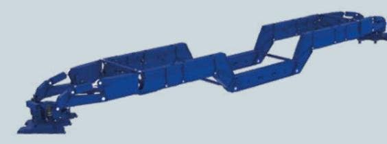
» With a payload of 350 t, the »FAKTOR« 5.5 high girder bridge can take on and transport up to 5,5 times its dead weight.
